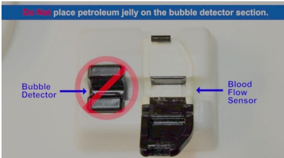
Figure 6. Bubble detector and flow sensor
